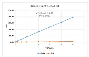
**Fig.2** High selectivity of GreenQuant dsDNA Kit for dsDNA over RNA. dsDNA and RNA from yeast samples (10  $\mu$ L) were assayed in triplicate with GreenQuant dsDNA kit. Fluorescence was plotted against the concentration of RNA or DNA. Background fluorescence had not been subtracted and the y-intercept was set at the RFU of the blank.
