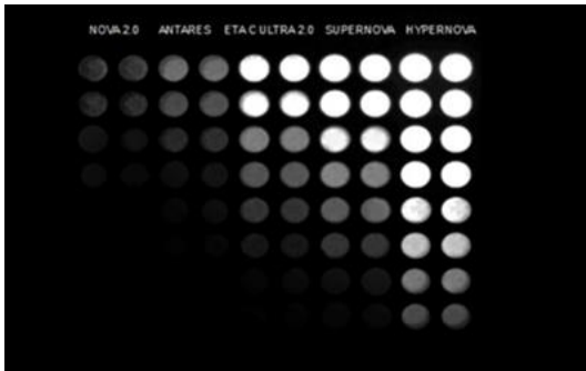
Figure 1. ELISTAR selection guide. Detection of 2-fold dilutions of HRP in a 96 microplate. Imager: ImageQuant™ LAS 4000 (GE Healthcare).
